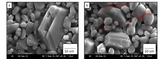
**Figure 6.** Scanning electron microscope of porous alumina when it was exposed to PZT at different magnifications showing large grain of lead.
