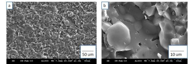
**Figure 5.** Scanning electron microscope of as-received alumina at different magnifications.
