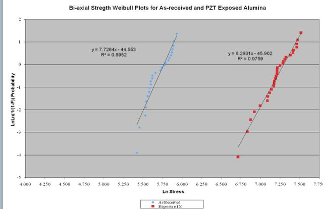
**Figure 3:** Weibull plot for as-received  $Al_2O_3$  specimens and when exposed to lead oxide vapor in the sintering furnace for PZT production.
