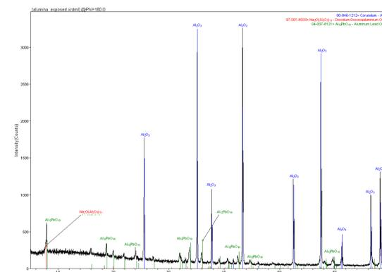
**Figure 4:** X-ray diffraction patterns of alumina when it was exposed to PZT.
