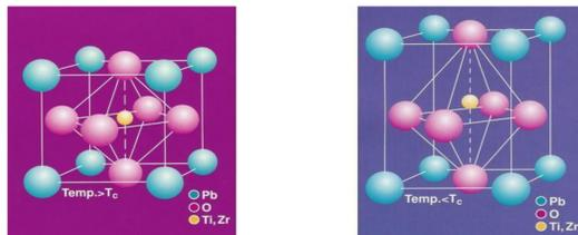
**Figure 1.** Crystal structure of cubic PZT changes during cooling. The crystal structure of PZT (a) above the Curie point the cell is cubic; (b) below the Curie point the structure is tetragonal with  $Pb^{2+}$  and  $Ti^{4+}/Zr^{4+}$  ions displaced relative to  $O^{2-}$  ions.<sup>1</sup>
